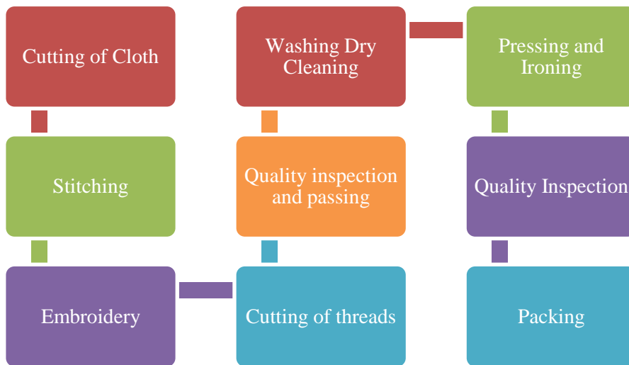
Figure 39 Process flow of apparel manufacture industry
