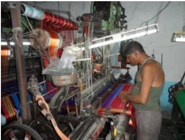
Ilkal saree weaving process in a power loom
